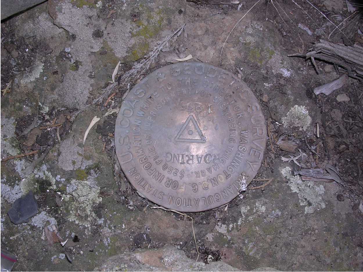
Figure 4.14 U.S. Coast & Geodetic Survey Roaring Springs triangulation datum.
